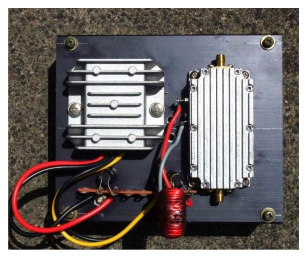
Photo shows a 15W amplifier and DC to DC converter mounted on a 155 x 130 x 50mm heatsink. The 30W amplifier is currently mounted on overly large heatsink as I had no idea how much heatsinking it would need.
